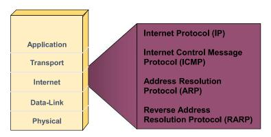
• In the OSI reference model, the network layer corresponds to the TCP/IP Internet layer.
