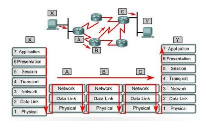
Data flow in a network focuses on layers one, two and three of the OSI model. This is after being transmitted by the sending host and before arriving at the receiving host.
