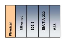
802.3 is responsible for LANs based on the Carrier Sense Multiple Access Collision Detect access methodology.
