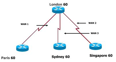
□In the example above, a /26 was used to provide the 60 addresses for Paris and the other LANs. There are no addresses left for WAN links
